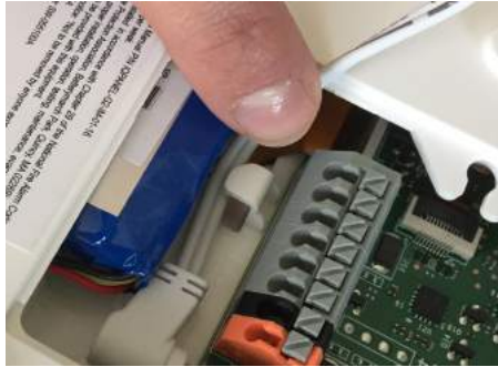
Route the wire behind the retainer clip
