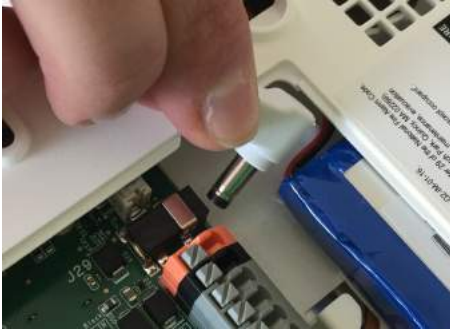
Plug in the power connector
