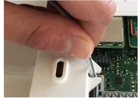
Insert the wire into the strain-relief
